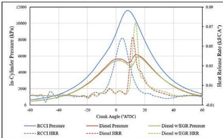
Figure 2: In-Cylinder Pressure and Heat Release Rate from RCCI and Conventional Diesel Combustion
