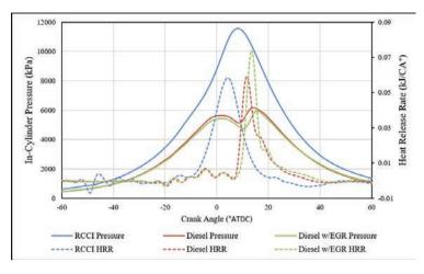
Figure 2: In-Cylinder Pressure and Heat Release Rate from RCCI and Conventional Diesel Combustion
