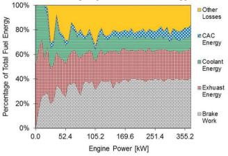
Figure 1: Energy Audit from 13 L HD Diesel Engine [4]
